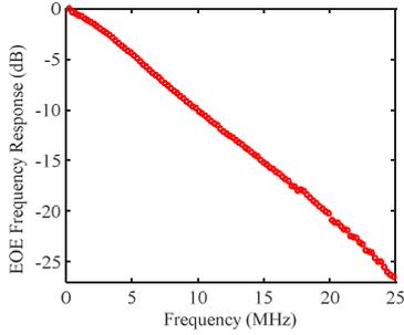
Fig. 3. The measured frequency response of the VLC system.
