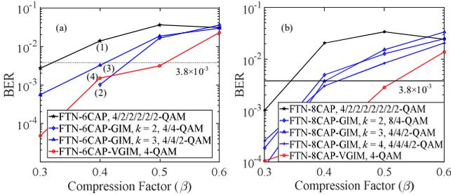
Fig. 4. Experimental BER vs. compression factor for FTN- $m$ CAP, FTN- $m$ CAP-GIM and FTN- $m$ CAP-VGIM with (a)  $m = 6$  and (b)  $m = 8$ .
