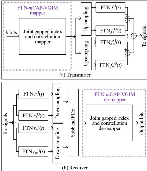
Fig. 1. Block diagram of the proposed FTN- $m$ CAP-VGIM: (a) transmitter and (b) receiver.
