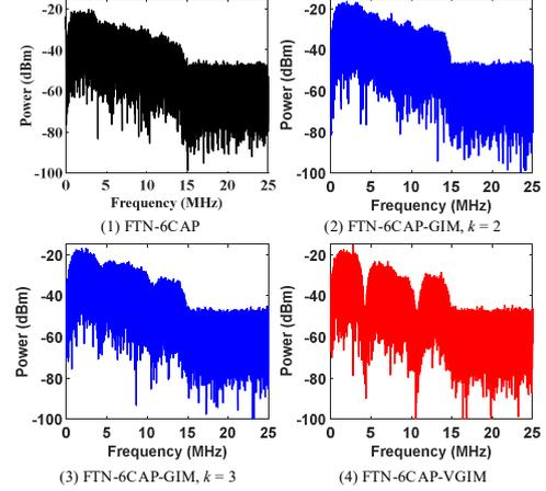
Fig. 5. Received spectrum of different schemes with  $m = 6$  and  $\beta = 0.4$ .
