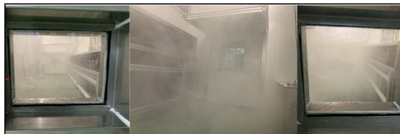
300*300mm coated glass (Transmittance \geq 95\% for 900-1600nm laser)
